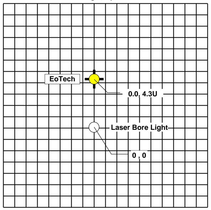
Zero Target Data for M16A4/M4MWS
